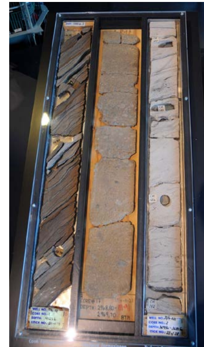
Core samples from the Statfjord field
