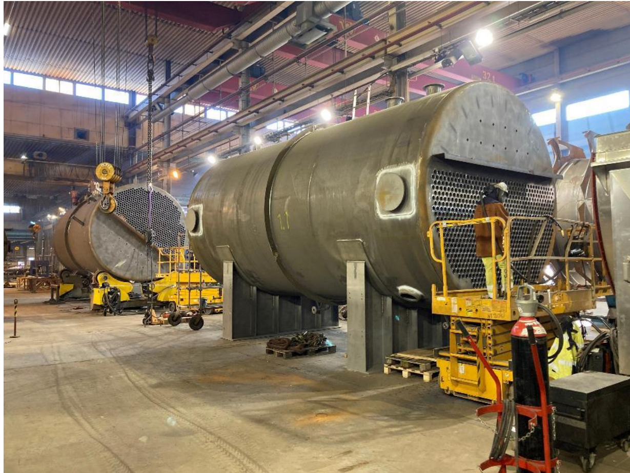
WRHU's being welded
