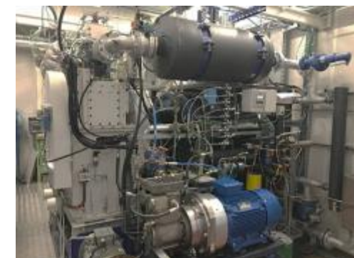
Single cylinder medium speed engine 1VDS 18/15 © LKV Rostock
