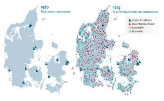
The Danish power system. Dominated by central power stations in the 1980s and today changed into a de-centralised power system with large amount of wind and solar power
